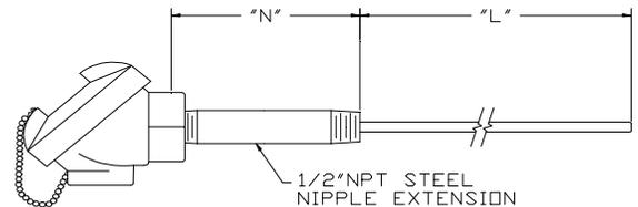
Model No. **M42** — Cast Aluminum Head w/ Steel Nipple-Union-Nipple Extension
