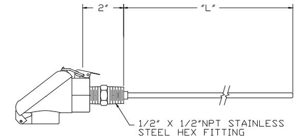
Model No. **M47** — Cast Aluminum Head w/ Steel Nipple Extension
