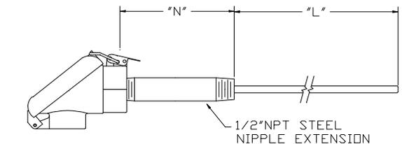
Model No. **M48** — Cast Aluminum Head w/ Steel Nipple-Union-Nipple Extension
