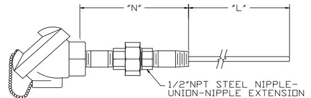
Model No. **M43** — Cast Aluminum Head w/ Steel Nipple-Union Extension
