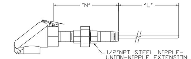
Model No. **M50** — Plastic Head w/ Stainless Steel 1/2" X 1/2" NPT Hex Fitting ( FDA Approved )
