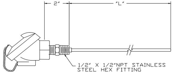
Model No. **M41** — Cast Aluminum Head w/ Steel Nipple Extension
